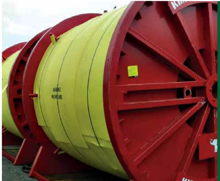
(Above and below) 90 metric ton reels of 3" diameter wire rope for the world's largest Derrick Lay Barges, such as DB101 and Semac 1. Ordered by KTL Offshore to the latest international standards.
