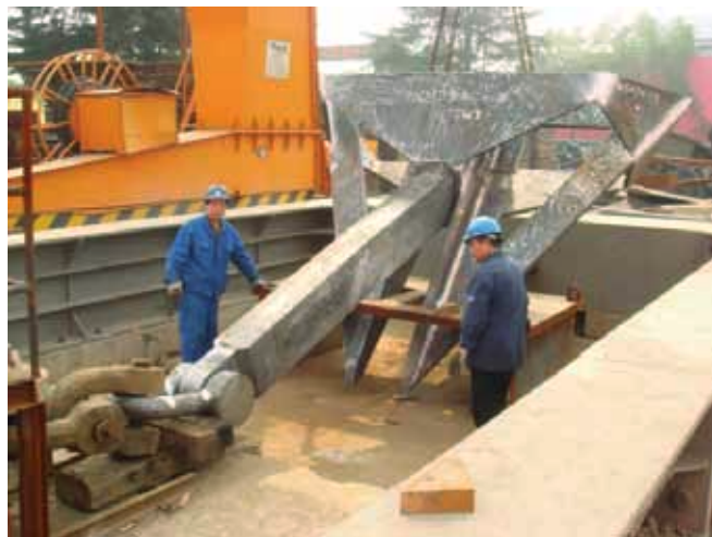
(Above) Anchors are made in China with 3 rd party inspection and witness of testing from Singapore.
